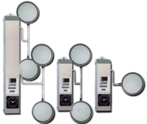
The MIKRO micro aerator offers you the highest quality of your cooling lubricant by introducing atmospheric oxygen. The floating air bubbles supply the cooling lubricant with oxygen and carry the impurities to the surface.
