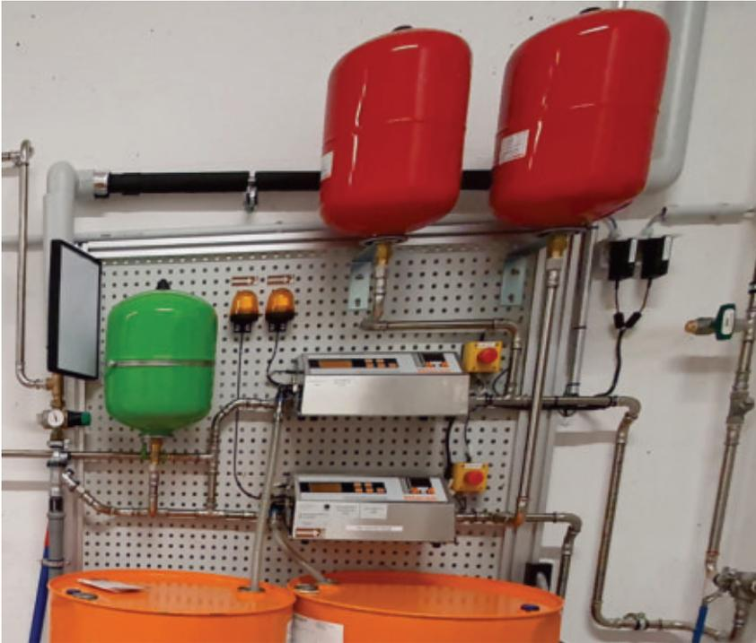
The mixing station is the heart of the automatic cooling lubricant filling.
